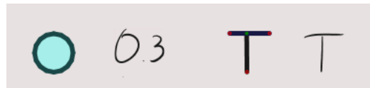
Figure 4. Text/drawing disambiguation. A leading ‘0’ or the initial stroke of a ‘T’ requires a 500ms delay during which an additional text stroke must be input.
