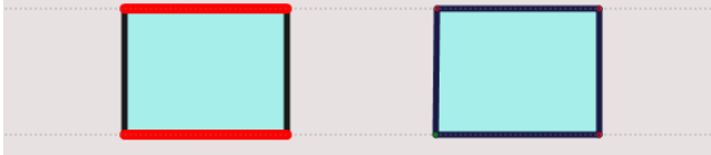
Figure 17. Construction lines. Two construction lines are created from the left rectangle by tapping to select its bottom and top edges. Subsequent drawing lines may snap to the construction lines.
